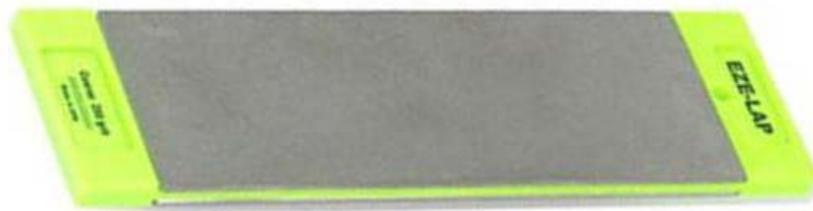
Good quality modern day knives have steel that is so hard that diamond plates with their greater cutting power are preferred to the softer aluminium oxide or silicon carbide stones. Good quality diamond plates, although more expensive, don't break, chip or hollow out like aluminium oxide and silicon carbide stones, and will last a lifetime.
